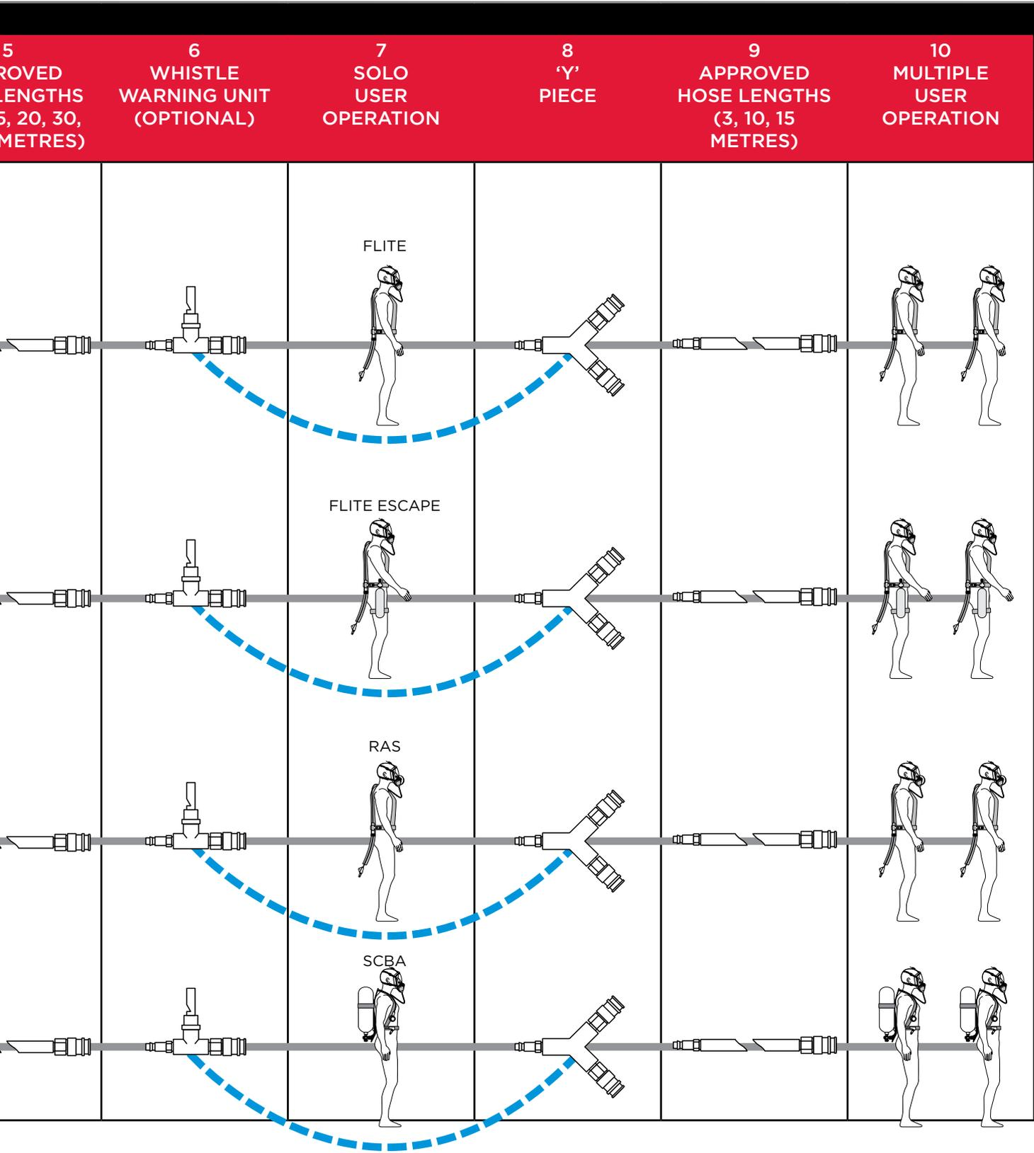
PLEASE NOTE THAT MANY OTHER CONFIGURATIONS CAN BE SPECIFIED. NB. THE LINE DRAWINGS ABOVE ARE ONLY REPRESENTATIONS OF SCOTT AIRLINE EQUIPMENT AND MODULAIR SHOULD BE NO MORE THAN 105 METRES. PLEASE SEE MODULAIR USER MANUAL FOR APPROVED CONFIGURATIONS.
