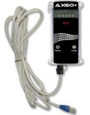
The Quick Connect Alarm is fitted with one cable gland and a 2-metre cable with a blue RJ45 connector. This should be connected to the Sensor which is associated with the Alarm, via an RJ45 coupler (or an RJ45 splitter if there is more than one Alarm).
