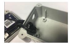
[4] Fit a gland blanking disc over the hole which the gland and cable were removed from.
