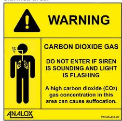
Again, an example label below, this label should be located next to the Central Unit and describes detailed  $CO_2$  alarm response procedures in UK English. Sensor locations and emergency telephone numbers must be added by the end user.
