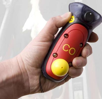
This unit is ideal for spot checking levels of carbon monoxide to ensure the wellbeing of humans and animals. Raised levels of this colourless, odourless gas could be as a result of poorly maintained brooders or another source of poor combustion. This ergonomically designed unit can easily be taken "point to point" and can even be bump tested with your breath so is simple to maintain.
