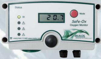
The Safe Ox is a single point O<sub>2</sub> enrichment monitor with a O<sub>2</sub> sensor which can last up to a decade! The Safe Ox includes a main unit for inside the room with the danger gas and a remote repeater alarm which goes outside the main entrance to the room so staff and visitors know if its safe to enter or not. Both parts give audible and visual warnings of a potential leak and the unit can be fitted with a battery back up and outputs such as: 4-20mA and relays
