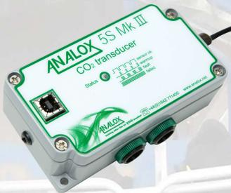
The 5S3 is a dual beam IR (Infra Red) CO<sub>2</sub> sensor which is ideal for monitoring CO<sub>2</sub> levels inside the silo bins to help prevent spoilage. The 5S3 is supplied in an aluminium enclosure, has a 5 wire connection and can offer 4-20mA or 0-2V output. This sensor can be linked to our MCU control panel to provide displays, alarms and datalogging.
