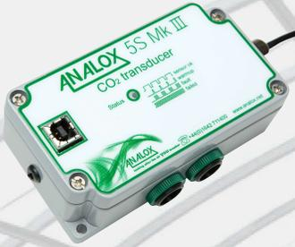
The 5S3 is a dual beam IR (Infra Red) CO<sub>2</sub> sensor which is ideal for monitoring CO<sub>2</sub> levels inside the glass house to ensure the best possible conditions for the yield. The 5S3 is supplied in an aluminium enclosure, has a 5 wire connection and can offer 4-20mA or 0-2V output. This sensor can be linked to our LC Commercial control panel to provide displays, alarms and outputs.
