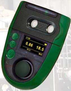
The "Livestock Aspida" can be cited at animal level and give continual readings of CO<sub>2</sub> & NH<sub>3</sub> and audio visual alarms should permissible levels be exceeded. The unit also datalogs and information easily retrieved through a USB connection. It can be used as a portable or fixed monitor.
