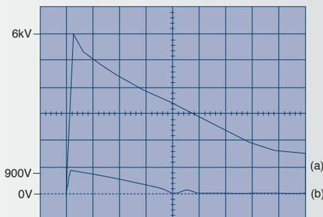
(a) BS6651:1999 Annex C open circuit voltage wave 6kV 1.2/50 $\mu$ s.
