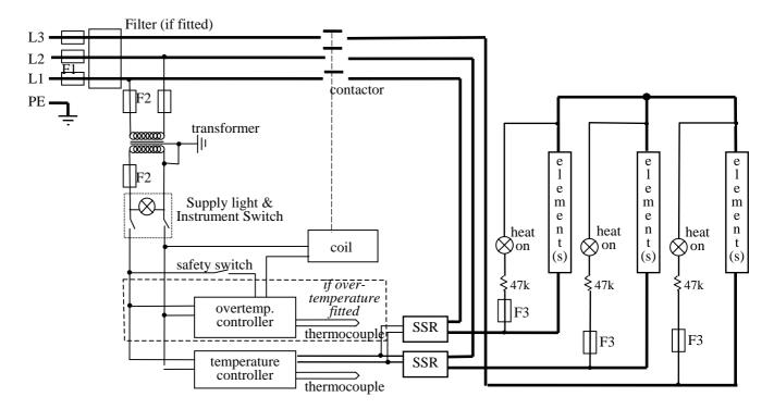
In this configuration the fuses F2 on the supply side of the transformer may be GEC Safeclip, not  $32 \times 6$ mm glass as stated in section 8.1.
