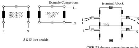
CWF /23 element connection example (1-phase 200-240V)
