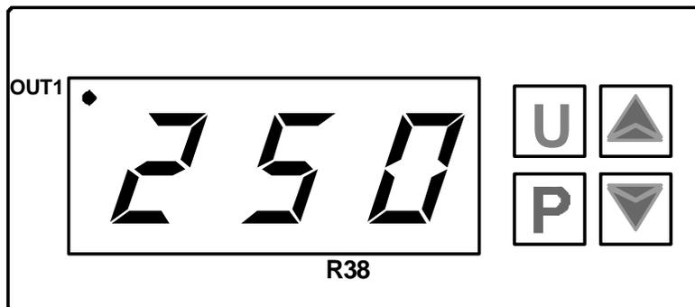
When switched on, the controller lights up, goes through a short test routine, and then displays the measured temperature and starts to control. The output light OUT1 indicates when heating is occurring.
