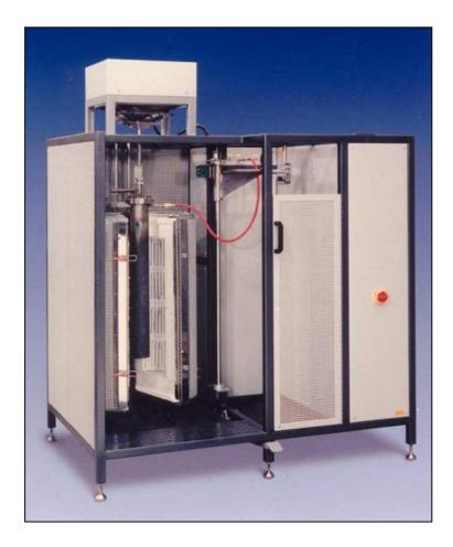
ASTM D 5341-93a Method for Measuring Coke Reactivity Index (CRI) and Coke Strength after Reaction (CSR).
