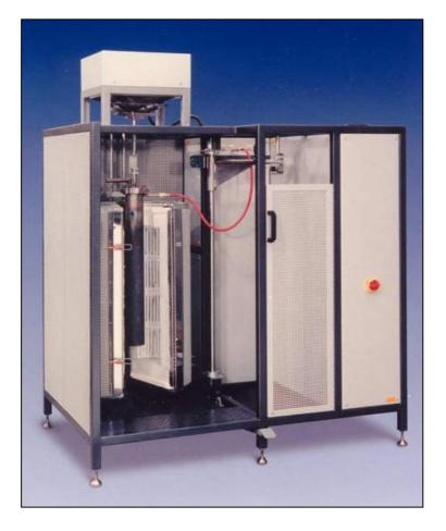
ASTM D 5341-93a Method for Measuring Coke Reactivity Index (CRI) and Coke Strength after Reaction (CSR).
