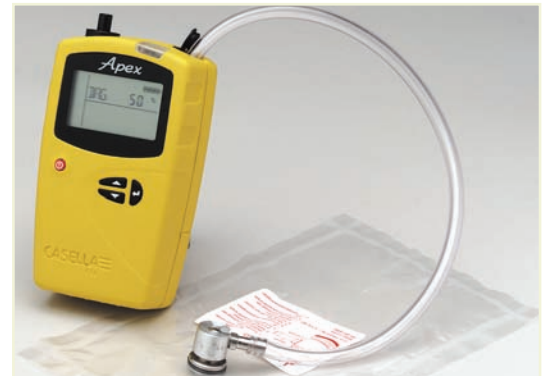
Pump with Tedlar gas bag for grab sampling
