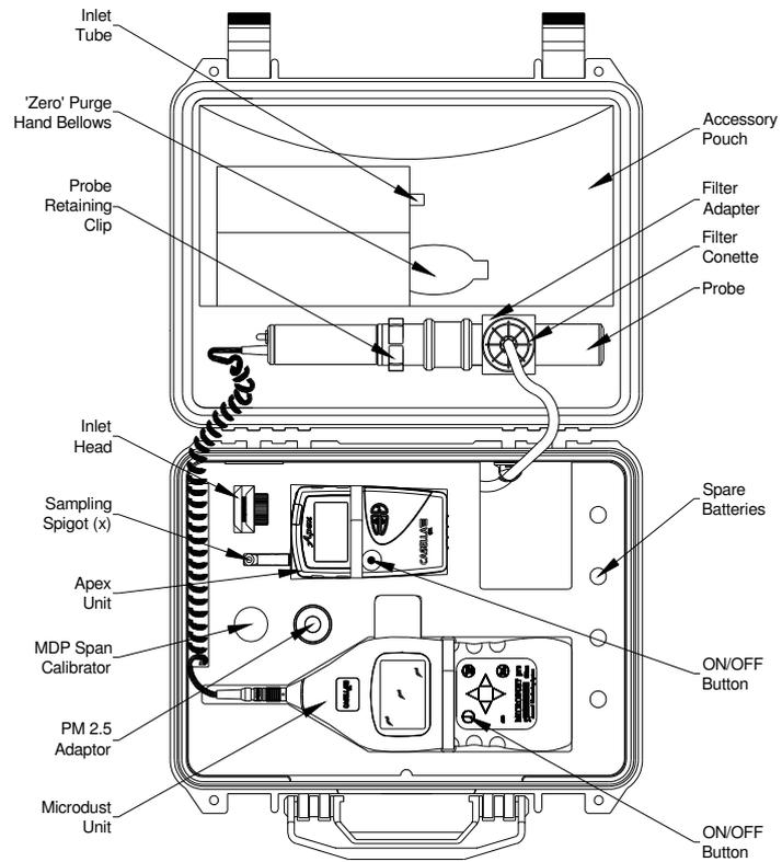
**Figure 1 - Components and controls for dust detective.**
