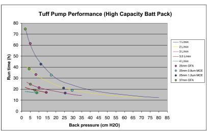
The **TUFF** pump incorporates a proven efficient double acting diaphragm pump mechanism with precise digital control. This offers the user excellent real time flow control and stability across a wide range of sampling media.
