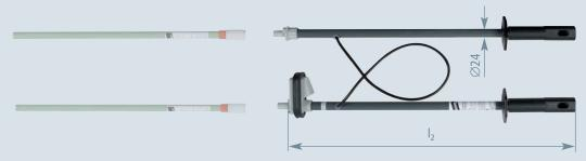
The two-pole PHV phase comparator consists of a test unit and two test prods which are attached to the test unit (to be ordered separately). To avoid confusion, the test prods have different colours according to the nominal voltage.
