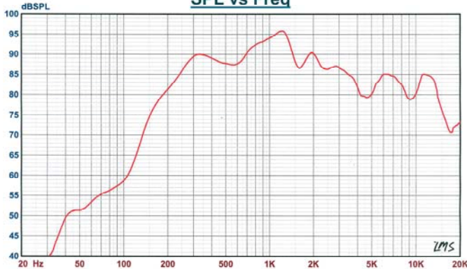
SPL at 1W/1m Sine wave SPL vs Freq
