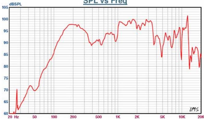
Sound pressure levels at 1W/1m P-6/15B
