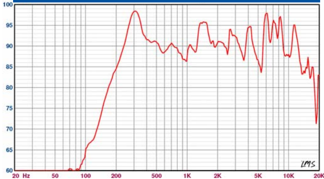
Sound pressure levels at different frequencies at 1W/1m P-5/15B
