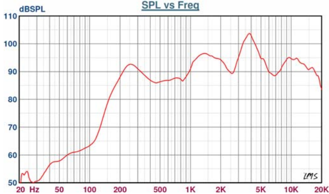
Sound pressure levels at 1W/1m P-5/15B
