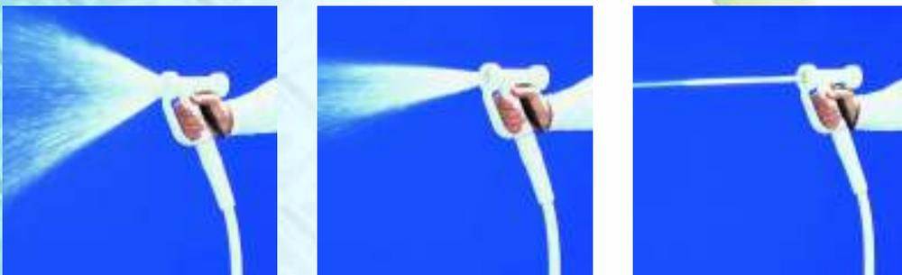
The operator can change the water pattern simply by adjusting the trigger position. A partial squeeze gives a wide drenching spray, for wetting large surfaces. The spray can be narrowed by applying a further squeeze. A full squeeze produces a concentrated jet, which is more effective in removing stickier and heavier substances.
