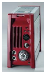
Integrated superior thermoelectric gas cooler, with automatic controlled water removal and easy field replaceable. The Cooler is able to drop temperature down to 5 C for moisture drop-out.
