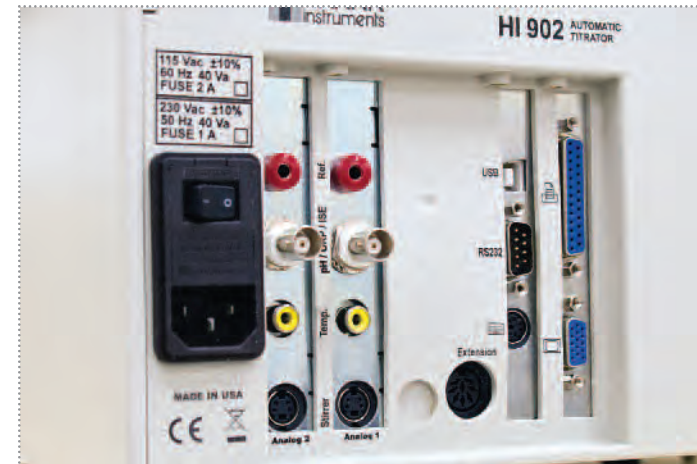
Support for 2 electrodes, 2 burette dosing pumps and 2 stirrers
