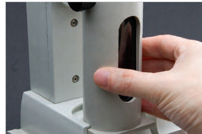
Clip-Lock™ Exchangeable Burette System
