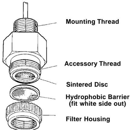
**Figure 1 Type 705 Sensor and Filter Housing**
