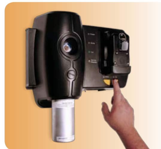
Calibrating QRAE II with AutoRAE Lite Bump Test and Calibration Station
