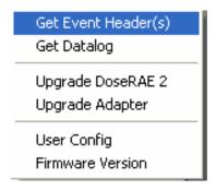
This menu is divided into three sections. The first allows you to Get Event Header(s) or Get Datalog. This means you can either get a list of events stored in the datalog or the complete datalog. If you select either one, it must download from the DoseRAE 2 to your computer.
