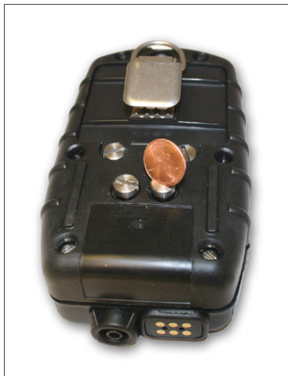
Figure 13. Loosening rear screws.
