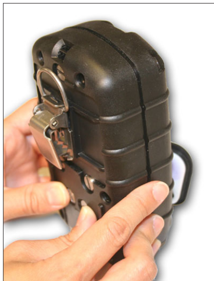
Figure 14. Pushing screws to remove sensor cover.
