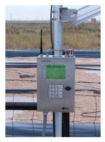
The FMC-2000 controller can monitor up to 24 wireless MeshGuard detectors and contains five programmable relays that can trigger external alarms or process controls.
