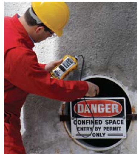
Confined space testing with the MultiRAE Lite
