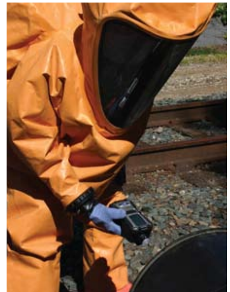
CBRN detection with the MultiRAE Pro
