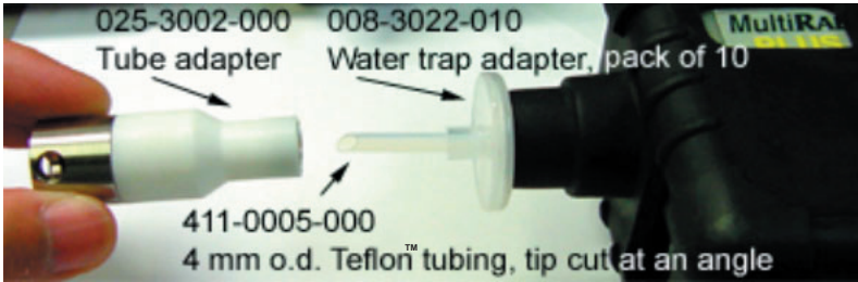
Connection to Multi-gas monitors
