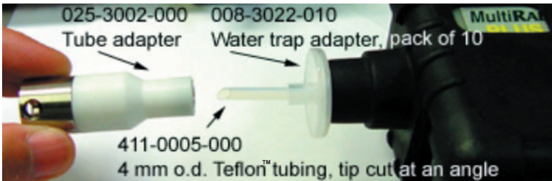
Connection to Multi Gas monitors
