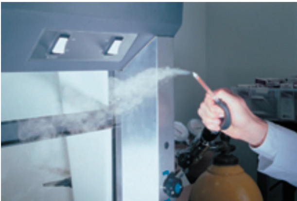
Figure 6.1. Use of smoke tube for visualizing fume hood air currents.
