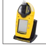
Integral pump and battery charger
