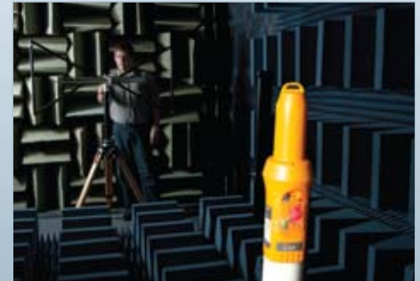
RF Anechoic testing chamber
