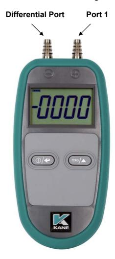
Always use the top right hand port (Port 1) for taking single channel measurements (pressure or vacuum). Only use the left hand port for differential measurements.
