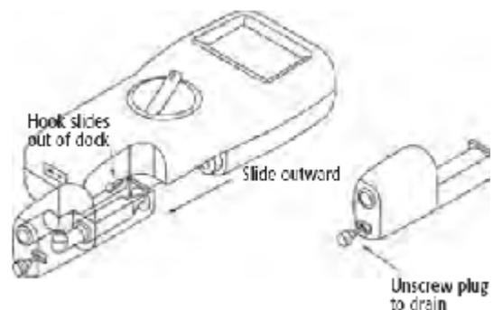
NOTE: O<sub>2</sub> reading will be invalid if the Water Trap Plug is not in place.
