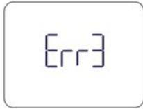
The monitor is measuring temperature outside its measurement range.
