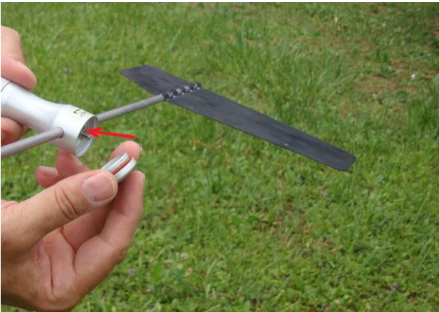
Fix the nut and fix the top (indicated by the arrows) and tighten it .
