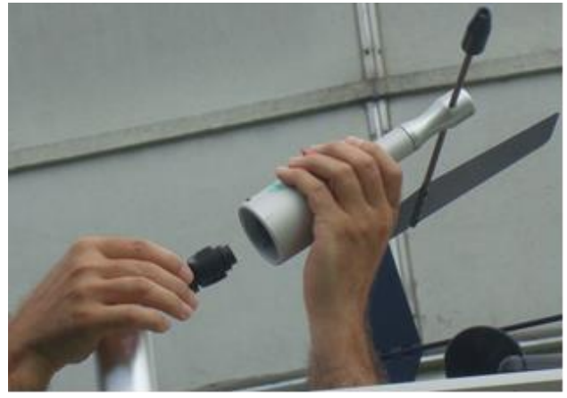
Connect the cable to the sensor.
