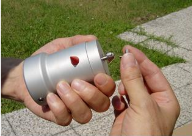
Unscrew the screw from the shaft thread.
