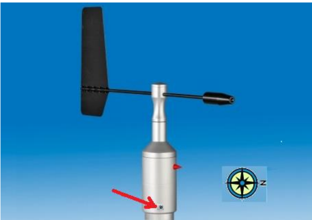
Mount the sensor on the mast and tighten the screw. When fixing the sensor in its position on the pole, point the "red nose" to NORTH for orientation.
