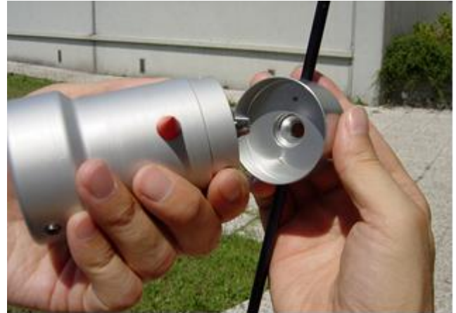
Insert the wind vane on the sensor's body. Take care to centre the wind vane's notch with the tooth on the sensor body's rotating cone.
