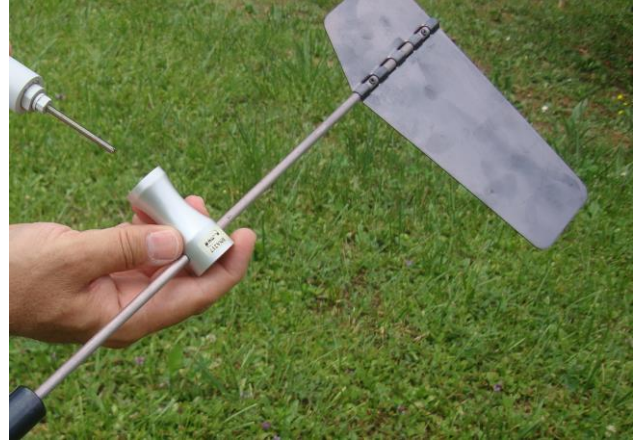
Insert the wind vane on the sensor’s body. Keep the shank in a steady position and insert the vane until it goes until the nut adjustment.
