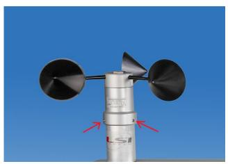
Mount the sensor on the mast and tighten the screws (indicated by the arrows).
