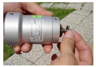
Unscrew the screw from the shaft thread.
