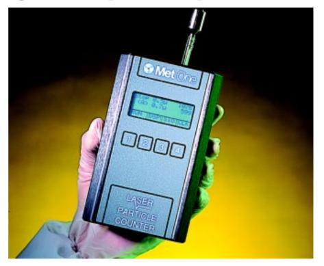
The Model 227 Portable Airborne Particle Counter offers the features and sensitivity of larger instruments and easy handheld operation. Weighing only two pounds, the Model 227 features a sensitivity of 0.3 micron (227B) or a sensitivity of 0.5 micron (227A), is fully self-contained, and uses reliable laser diode technology. It connects to a remote printer or computer, and can be part of a facility-monitoring system.
