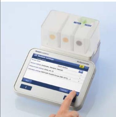
The instrument provides calibration support on many levels, featuring methods with a fixed calibration sequence, automatic evaluation of the calibration results with optional rejection and monitoring of the sensor's age and calibration interval. Automatic calibration with the Rondolino sample changer is also possible!
