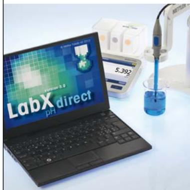
The LabX direct pH PC software allows for easy and efficient export of results during analysis. The transfer settings for this software need to be activated only once in the instrument and will work automatically with plug-and-play.
