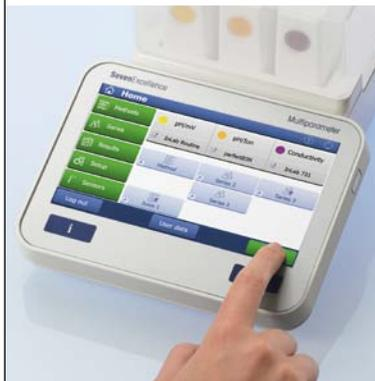
This instrument encompasses a second possibility to start a measurement or calibration by pressing READ or CAL. Although more flexible, performing direct measurements in a row with varying parameters requires a change of settings before each sample.
