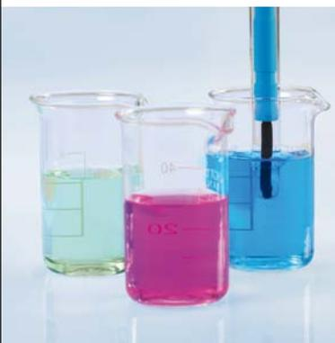
Using methods is a secure and efficient way of calibrating a pH sensor. Once a method is created, each calibration will use identical settings. Limits for offset and slope can be monitored to avoid a poor calibration from being stored.
