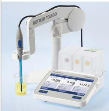
uPlace™: the electrode arm can be operated with one hand, moving perfectly straight up and down to bring the electrode in the perfect position. This allows for faster measurements and poses less risk of the sample vessel tipping over and damaging the sensor!
