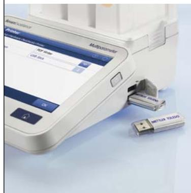
Users wishing to document results have an alternative to printing the data on a METTLER TOLEDO or network printer, as the instrument also supports exporting results in pdf format to a memory stick. This is especially interesting for a paperless laboratory.
