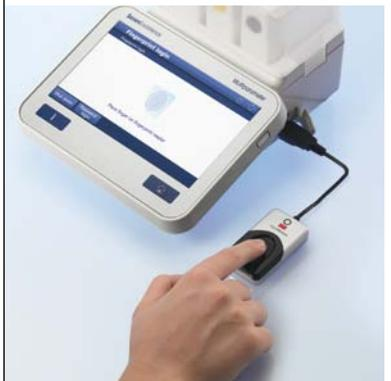
In addition to typing a password, the instrument also supports the LogStraight™ external fingerprint reader. This not only offers a convenient login solution, but also provides an extra degree of security!
