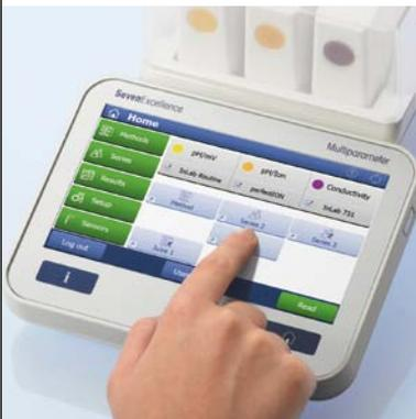
By a single click on a shortcut you can start a method: a sequence of analysis steps with fixed pre-set parameters. Using methods makes sure that your particular analysis is always performed with identical settings.
