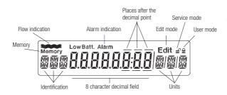
Meter readings with up to 8 numerical characters, symbols and short texts can be shown on the multifunction display as an interactive process guide.
