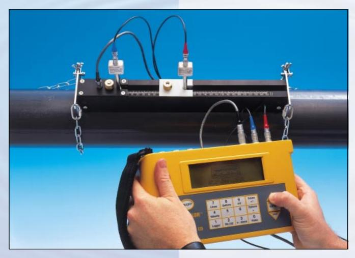
**The Portaflow** 300 can be applied to both clear and cloudy liquids in any type of pipe including those with composite walls. It is user friendly, compact, lightweight and thanks to modern technology, low cost, both to purchase and operate.
