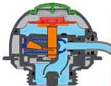
AutoMaXX® with positive pressure – valve open
