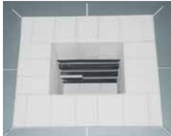
Two-Side heating with SiC rods
