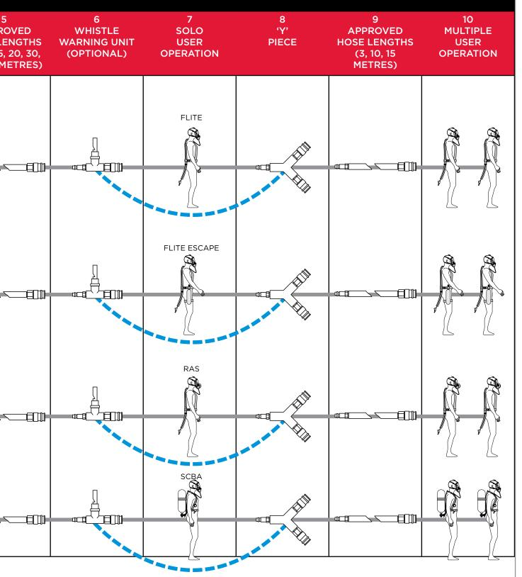
SE NOTE THAT MANY OTHER CONFGURATIONS CAN BE SPECIFIED. NB. THE LINE DRAWINGS ABOVE ARE ONLY REPRESENTATIONS OF SCOTT AIRLINE EQUIPMENT AND DULAIR SHOULD BE NO MORE THAN 105 METRES. PLEASE SEE MODULAIR USER MANUAL FOR APPROVED CONFIGURATIONS.
