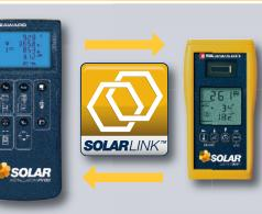
Solarlink™ connectivity enables irradiance to be displayed and for irradiance, module and ambient temperature to be recorded with the PV150 (available separately) in real time as electrical tests are conducted.
