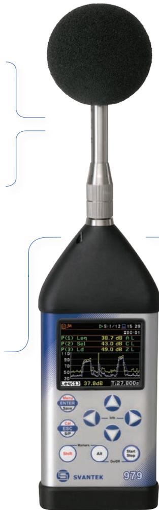
When dealing with **facade insulation** it is often necessary to evaluate the background noise on the building surroundings. The effective and low-cost solution to this requirement is a waterproof portable monitoring kit set-up to do periodical measurements of the environment. When required, the SVANTEK instrument can be locked into the protective case and placed in a suitable position for outdoor noise measurement.
