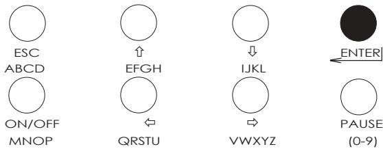
The **ENTER** key allows the operator to accept any entry and move onto the next data entry field or screen. It also starts a program in Program Mode.
