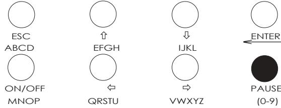
Except when the Ramp Rate is set the MAX, the **PAUSE** key allows the operator to pause the unit (a 'P' will appear on the display) until the PAUSE key is pressed again (the 'P' will disappear) or until the ON/OFF key is pressed to stop the Calibrator. Where a word can be entered, then successive presses of this key will toggle through the numbers **0-9**.
