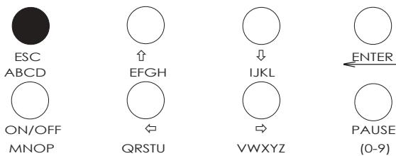
The **ESC** key allows the operator to exit the current sub-menu and go back to the next higher level menu. Where a word can be entered, then successive presses of this key will toggle through the letters **ABCD**.
