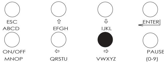
The  $\Rightarrow$  key allows the operator to move within the data field. Where a word can be entered, then successive presses of this key will toggle through the letters **VWXYZ**.
