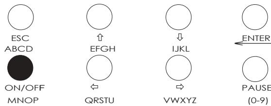
The **ON/OFF** key allows the operator to start or stop the unit in Manual Mode or stop a program in Program Mode. Where a word can be entered, then successive presses of this key will toggle through the letters **MNOP**.
