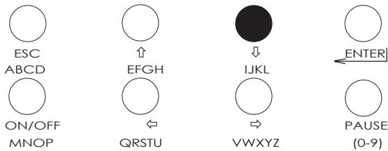
The **↓** key allows the operator to move down the current sub-menu. This key can also be used to decrease numeric values in some fields. Where a word can be entered, then successive presses of this key will toggle through the letters **IJKL**.
