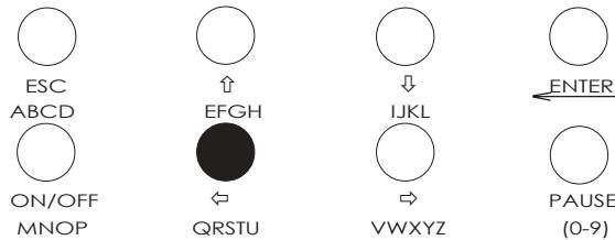
The  $\leftarrow$  key allows the operator to move within the data field. Where a word can be entered, then successive presses of this key will toggle through the letters **QRSTU**.
