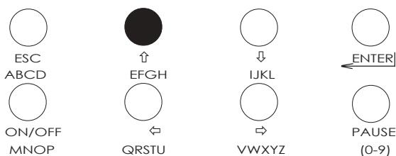
The **↑** key allows the operator to move up the current sub-menu. This key can also be used to increase numeric values in some fields. Where a word can be entered, then successive presses of this key will toggle through the letters **EFGH** until the **ENTER** key is pressed.
