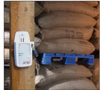
Monitors humidity and temperature values e.g. in warehouses
