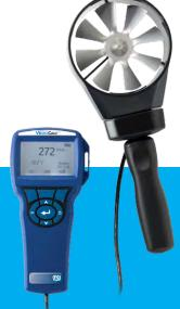
It accurately measures air velocity and temperature, calculates flow rate, performs averaging, and can determine minimum and maximum readings. Using sweep mode, you can quickly provide one averaged reading of velocity or volume over a large measurement area. The large vane head automatically averages and dampens velocity and volume readings. The VelociCalc 5725 includes variable time constant, sampling and statistics functions and data logging capability.
