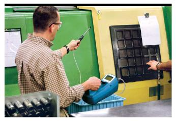
P-Trak Ultrafine Particle Counter and accessories includes: Telescoping Sample Probe, Shoulder Strap, Inlet Screen, Spare Wicks (2), Alkaline Batteries, Alcohol Fill Capsule with Storage Cap, Reagent Grade Isopropyl Alcohol, Zero Filters (2), Carrying Case, TrakPro™ Software, Computer Cable, Operation and Service Manual, Calibration Certificate, and Two-year Warranty.
