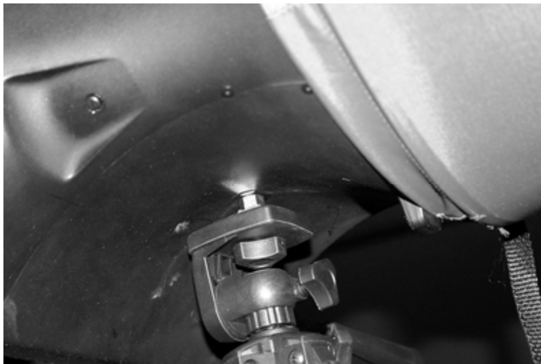
Figure 25: Mount Micromanometer Base to Telescopic Stand
