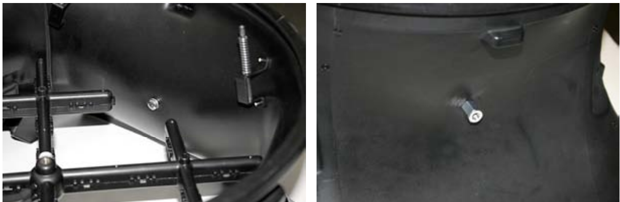
Figure 23: Remove Plug Located at Back of Base Assembly
