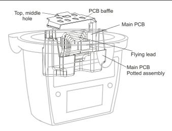
Push the communication board earth lead through the top middle hole in the baffle.
