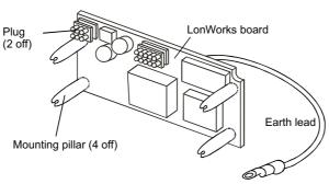
Note: The board is supplied with the mounting pillars fitted to it.
