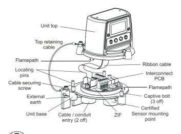
2. Disconnect the cable retaining the Transmitter Unit top to the base.
