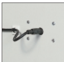
Rear view of cabinet door, showing simple plug-in connection for the cable running between the protector unit and the remote display.
